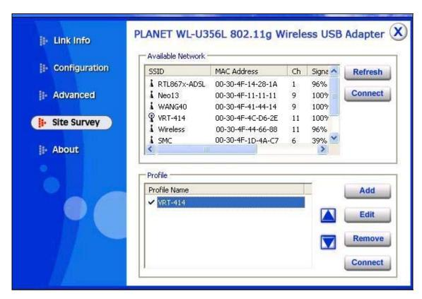
This screen shows the APs or Adapters which available for WL-U356L to connect. If you configure the SSID of WL-U356L as "Any", it will show all available APs and Adapters at the same time.
